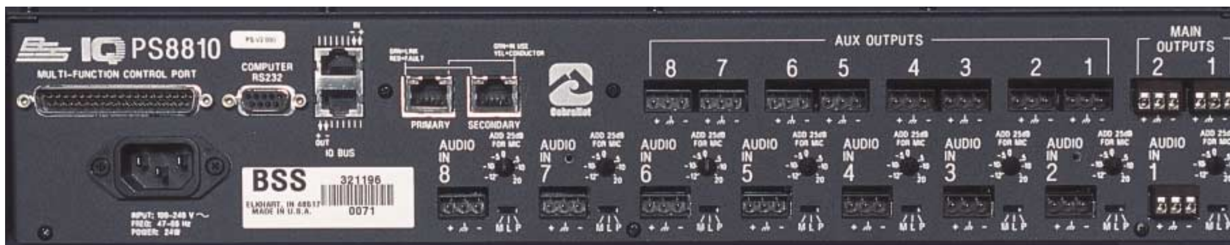
Rear Panel Controls: A 3-position selector switch (mic/line/phantom) and a calibrated gain control for each input.
